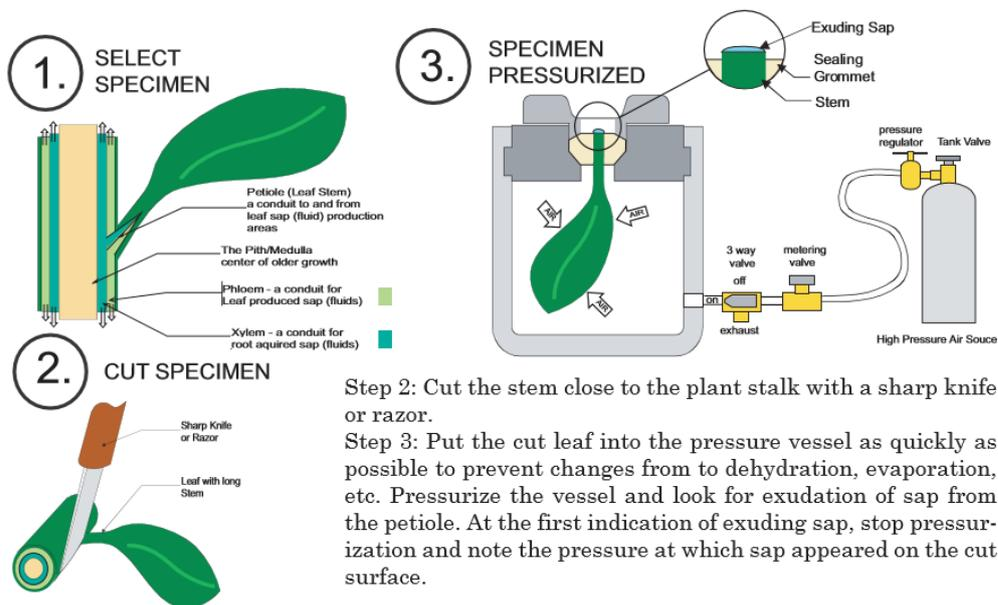
**A2.** Diagrammatic illustration of the use of the Pressure Bomb as per Soil Moisture Equipment Corp. (2006).
