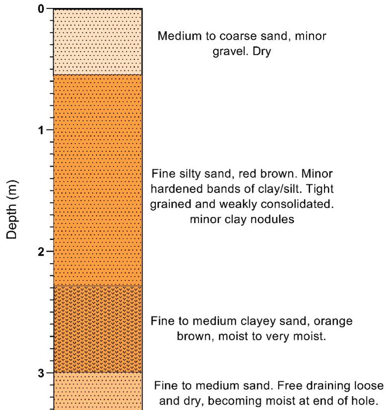
***End of Hole 3.5m - Abandoned due to collapse***
